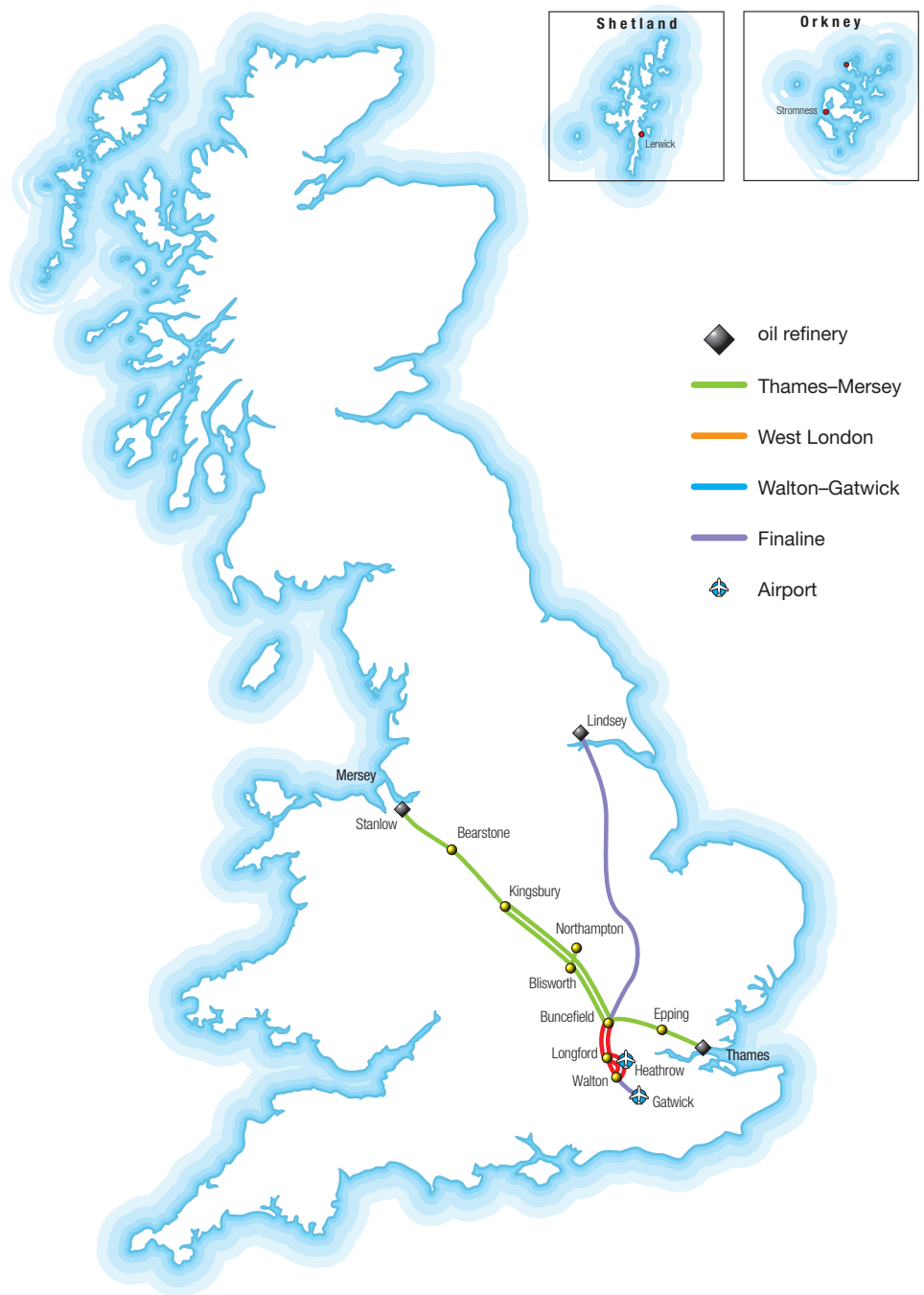
Figure 4 Schematic showing the pipeline system supplying Buncefield
