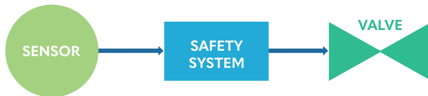
Figure 13. Safety instrumentation system with typical components
