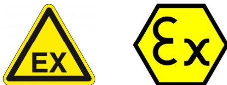
Figure 19. Triangle indicating ATEX zoned area and 6 corner (diamond) Equipment that can be used in a zoned area
